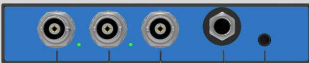
SDI In Alt SDI In SDI Loop Out AES/EBU In Analog Audio In
